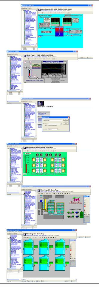
The Mimic module is the software equivalent to a hard-wired control panel offering comprehensive operator interfacing to your process control requirements.
