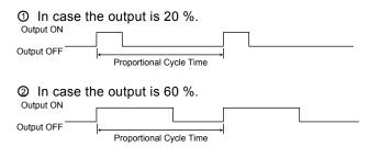
Output is ON during 20 % time of the proportional cycle time, and OFF during 80 % time of proportional cycle time.
